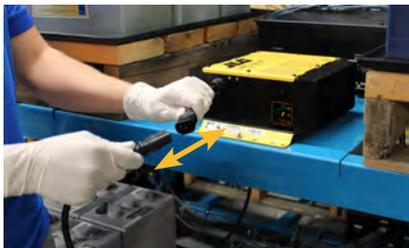
Figure 2: Disconnect AC power.
